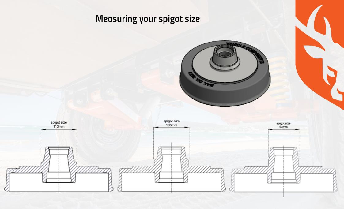
The spigot should be measured at its lower end where the spigot meets the drum face.
