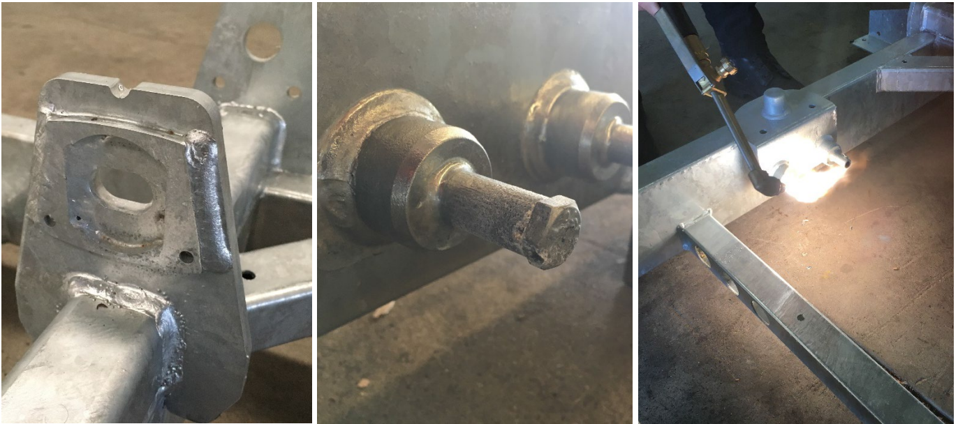
FIGURE 3: Buildup of gal coating on suspension mounts cleaned using heat
