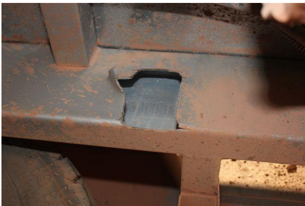
Figure 1: Chassis rail damage due to shock absorber outrigger being pulled off
