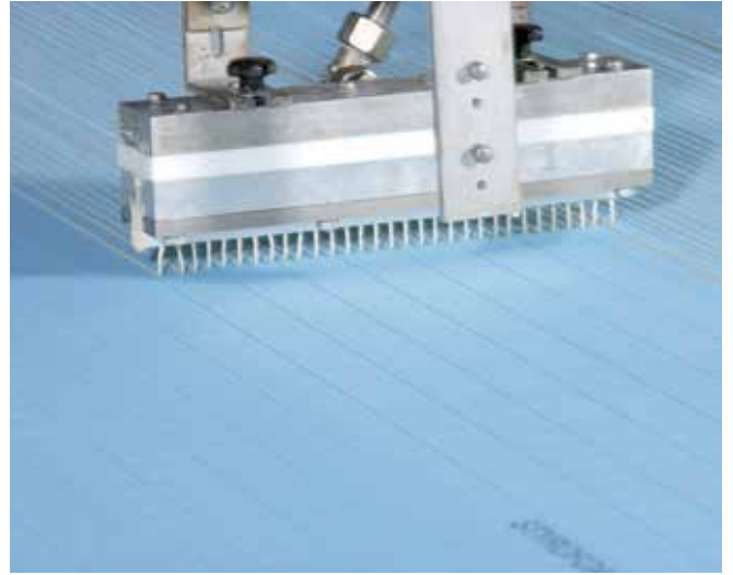
Fig. 11: Adhesive being applied to STYROFOAM™ core layer material
