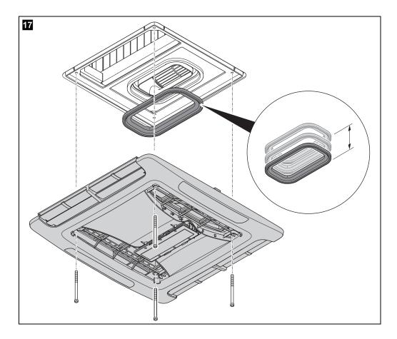
Stack the duct sections and place against the roof thickness: the duct height should match the roof height. Or use the below table as a guide:
