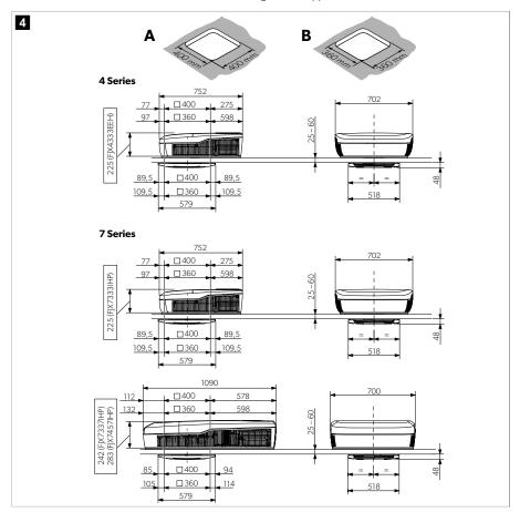
**3.** Mark the position and size of the opening  $(400 \times 400 \text{ mm})$ .
