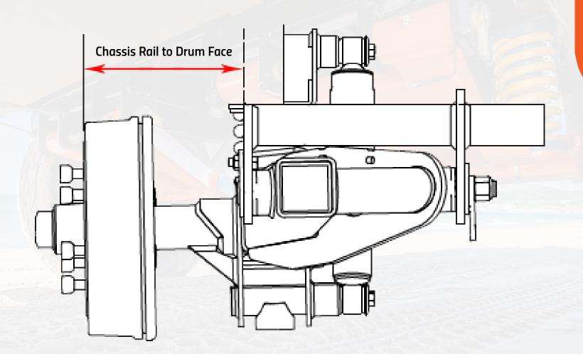
C/F is calculated by measuring from the outer drum face to the outer face of the chassis rail. An accurate C/F is vital in ensureing the wheel has the right amount of clearance when in motion.
