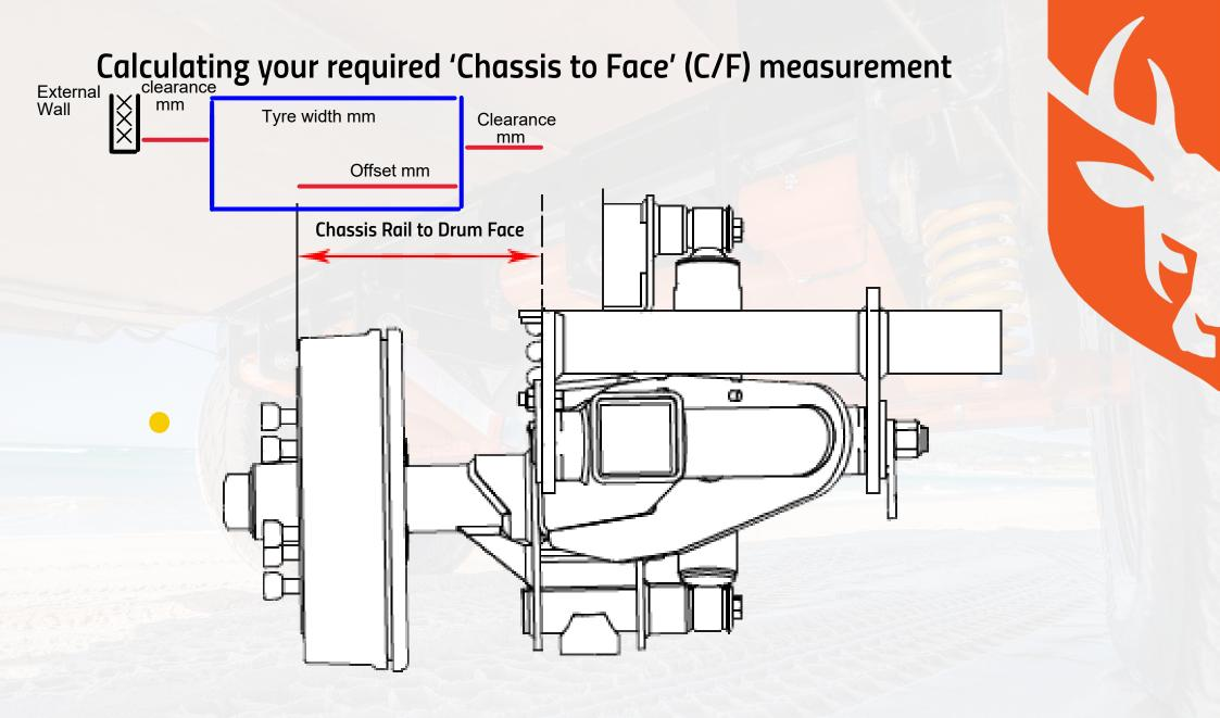
C/F is calculated by measuring from the outer drum face to the outer face of the chassis rail.
