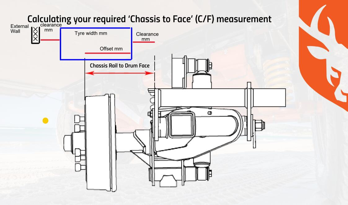
C/F is calculated by measuring from the outer drum face to the outer face of the chassis rail. An accurate C/F is vital in ensureing the wheel has the right amount of clearance when in motion.
