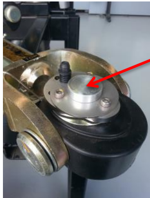
Bi-lock pin installed in DO35 coupling (Top View)
